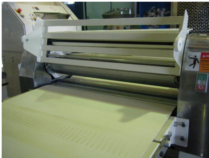
Fig1.7 Safety guard in the raised position
