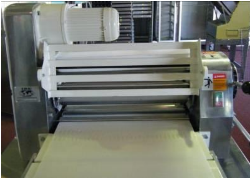
Fig1.7 Safety guard in the raised position
